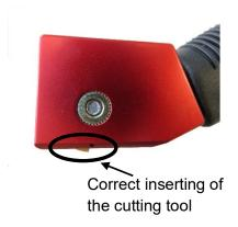
Refasten the fixing screw (4) with the Allen key.
