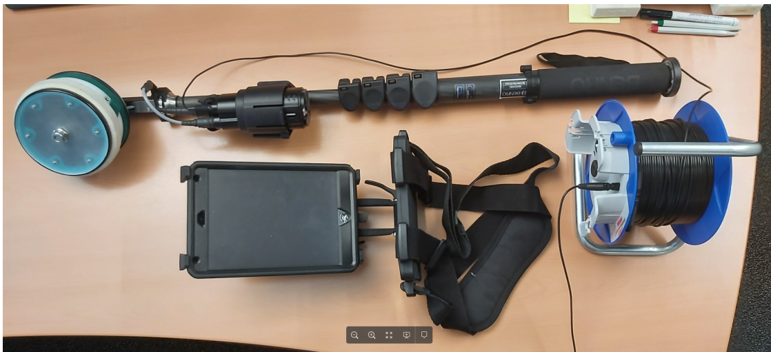
Figure 8 : PM8500 One wheel electrode cabling set up
