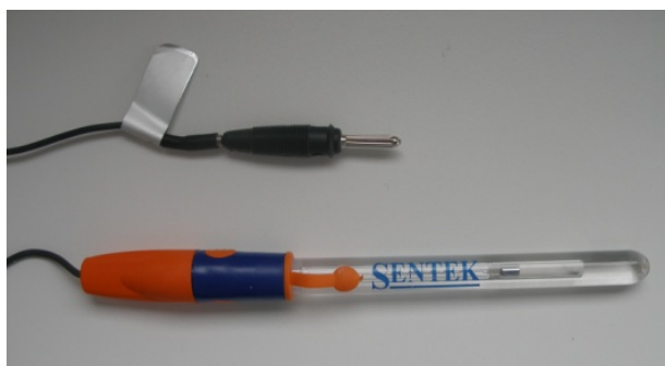
Figure 33 : Calomel (HgCl) Reference Electrode
