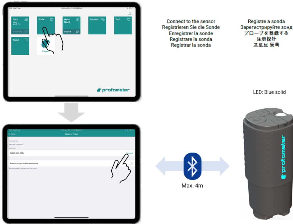
Figure 22 : PM8500 Profometer App: connecting the probe
