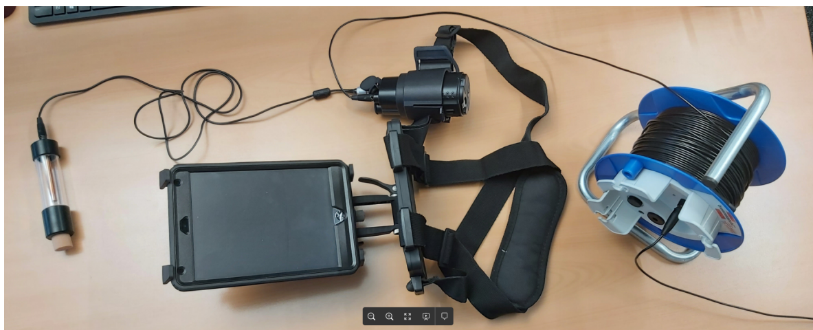
Figure 7 : PM8500 Rod electrode cabling set up
