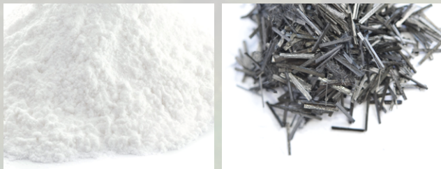
Materials used for carbon ceramic brake discs: silicon carbide and carbon fibers
