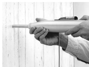
Fig. 5.2 Deploying the impact plunger (1)
