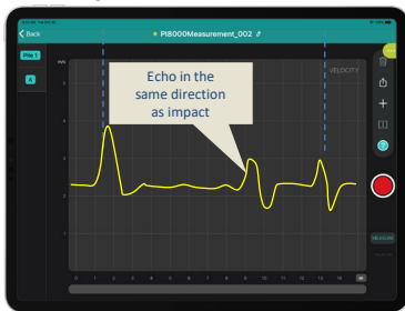
Necking – reduction in diameter
