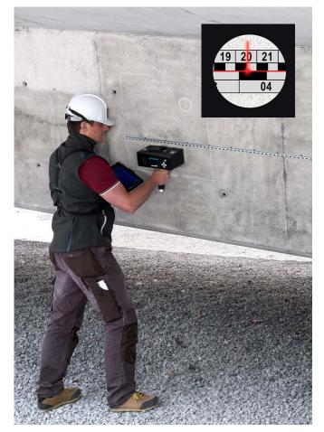
Positioning monitor showing the actual detected position
