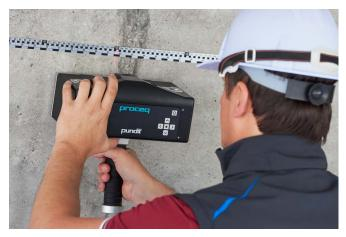
Error-free positioning with the Pundit Live tape measure
