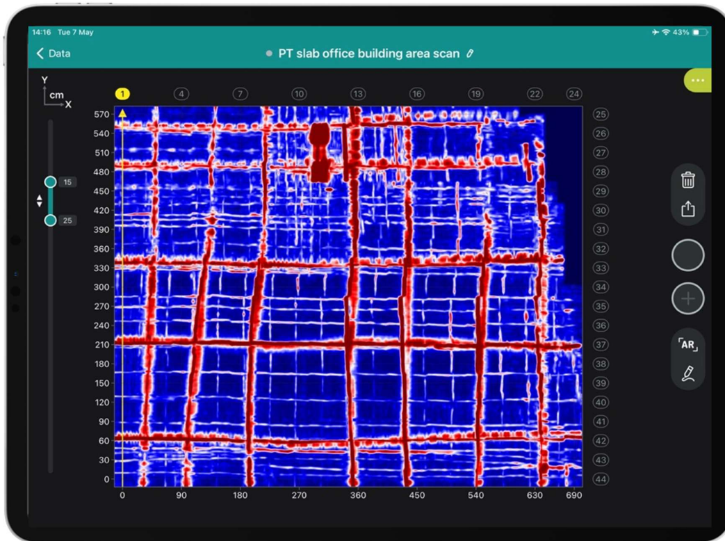
Figure 55: GP app software area scan PT concrete slab application
