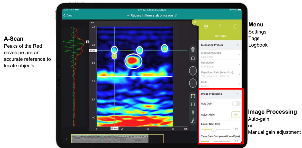
Figure 35: GP app software image processing auto-gain or manual gain adjustment
