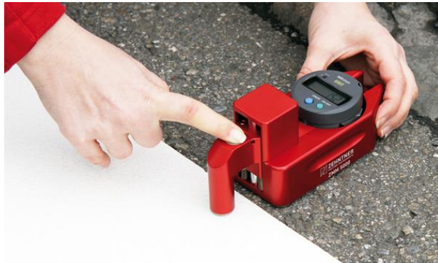
Figure 2: Placement next to the marking
