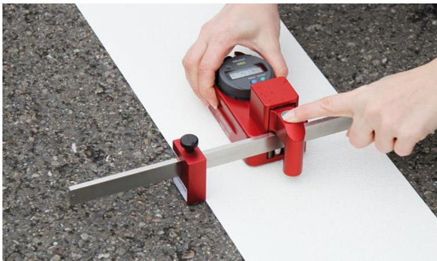
Figure 5: Placing with optional measuring bridge
