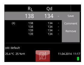
In case measurements are not stored automatically, the settings have been changed. This is described in chapter 14.3.2 "Auto save measurements" on page 48. Not stored measurements can be stored individually by choosing in the measure mode a single measurement and choose "Save".
