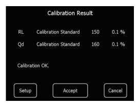
Press the symbol and to open the calibration function. In the standard setting there are listed night visibility RL and day visibility Qd to be calibrated on the calibration standard. If you wish to check the **ZRM 6013+**, you need to change the calibration settings. Press in the menu "Calibrate" the button
