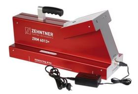
To charge the battery, plug in the charger plug on the **ZRM 6013+** and connect the charger to a wall socket (100 - 240 V, 50 - 60 Hz).
