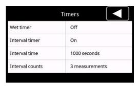
If the interval timer is activated, you can see the current setting for the interval time and interval counts. For changing these settings, you need to press the respective line.
