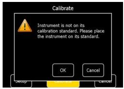
Take care that the ZRM 6013+ is placed correctly on the included calibration standard. Otherwise, the ZRM 6013+ will give you an error message. The instrument has to snap in which is indicated by a click sound.
