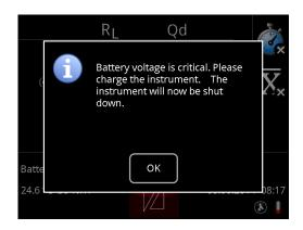
In order to prevent a damage of the battery, the instrument switches automatically off before the battery is completely empty. The **ZRM 6013+** announces this by displaying the symbol of an empty battery and an error message.
