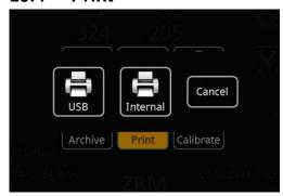
By pressing the button and you have the possibility to print out either the last measurement or a specific measurement earlier marked in the measure mode display using the optional built-in thermal printer or an USB-printer such as our optional portable printer. Without marking the last measurement will be printed. The default setting which information is included in the measuring report can be changed in the menu as described in chapter 14.6.8 "Printer" on page 58.
