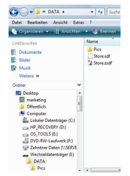
After the software has been recognised the Windows explorer might look as shown on the left side. You are able to make a back-up copy (the files Store.sdf, Store.zsdf and the folder Pics) on your local hard disk.
