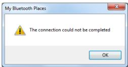
An error message will occur on your PC/laptop if the connection cannot be established. In this case check if the Obex service is activated on your PC/laptop. Right click on the Bluetooth® icon ® on the toolbar of your device (PC/laptop) and choose "Show Bluetooth Devices" and the tab "Services" and check "File Transfer (Obex)".
