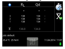
For activating average reading press on the touchscreen the symbol . If the symbol is shown, the average reading is activated.
