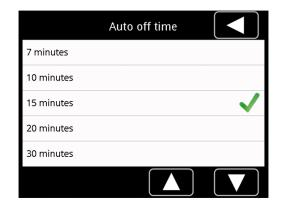
If there is no action the instrument will shut off once the "Auto off time" has been reached.
