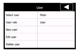
To add a user enables relating measurements to a specific operator and to store user specific settings. If no user has been added, the user "Peter" will be used for each measurement. The operator is shown on the bottom of the measuring report which can be printed. If you change any setting at a certain user this will be stored automatically at the user profile.
