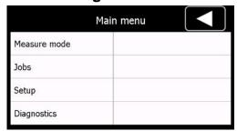
Press the button and to get into the menu where you can set different settings. Activate, deactivate, scroll and exit the menu as described in chapter 7 "Navigation" on page 16. On the top of each window you can read in which menu you are.
