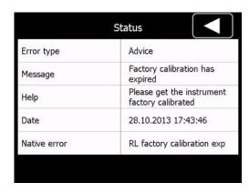
The instrument has been calibrated in the factory 2 years ago or even more time ago. It should be sent back to the manufacturer for checking, calibration and certification. Contact Proceq or your authorized Proceq-agent for returning the unit.
