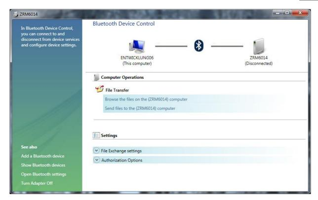
Click on "Browse the files on the (**ZRM 6013+**) computer". The **ZRM 6013+** is displayed like a USB-flash drive, and all common file and folder operations (move / delete / copy) are available. You might have to press "F5" to refresh the display.
