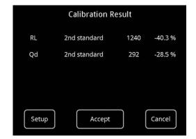
In order to prevent an unintentional calibration to completely wrong values (e.g. if the standard is damaged or soiled or the optic window on the bottom side of the instrument is soiled), you have the possibility to display the deviation in percent from the nominal value of the 2<sup>nd</sup> standard. By pressing and and selecting "Setup" and "Calibration" you can change these settings.
