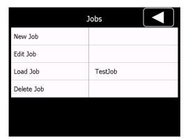
The **ZRM 6013+** offers the possibility to relate measurements to a specific job. Depending on the type of your company (contractor, road laboratory, manufacturer of road marking materials) a job could be a specific client, the development of product "xy" and so on.
