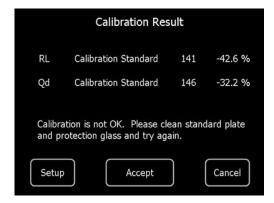
In order to prevent an unintentional calibration to completely wrong values (e.g. if the standard is damaged or soiled or the optic window on the bottom side of the instrument is soiled), the instrument tells you how much the calibration diverges from the nominal value.
