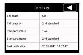
Afterwards you will be shown the information. The standard value needs to be consistent with the retroreflection values mentioned on the label which is on the backside. Adjust the standard value if necessary.
