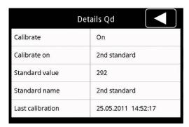
Please check the calibration settings also for the Qd geometry and if necessary change them accordingly.
