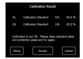
In order to prevent an unintentional calibration to completely wrong values (e.g. if the standard is damaged or soiled or the optic window on the bottom side of the instrument is soiled), the instrument tells you how much the calibration diverges from the nominal value.
