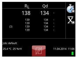
After a successful reading, the measurement values will be shown on the top.
