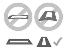
Make sure to use large enough, absolutely plane samples, insensitive to moisture, as e.g. sheet steel.
