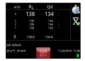
The single values are still displayed. On the left side of the page the measurements are numbered. On the bottom line you see the symbol for the average
