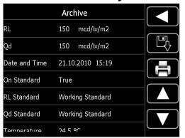
At a measurement entry you will find firstly the measuring values, the date/time and on which standard the instrument has been calibrated for this measurement or series of measurement respectively.
