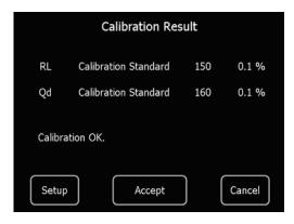
Press the symbol and to open the calibration function. In the standard setting there are listed night visibility RL and day visibility Qd to be calibrated on the calibration standard.
