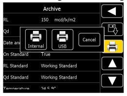
By pressing the symbol you are opening the window for selecting a printer. Here you can either choose the optional built-in thermal printer or an external printer connected to the USB-interface. By pressing the desired printer the measuring report will be printed out.
