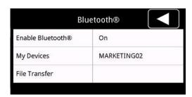
Prepare the **ZRM 6013+** for file transfer by pressing and and selecting "Setup" and "Bluetooth®" and "File Transfer".
