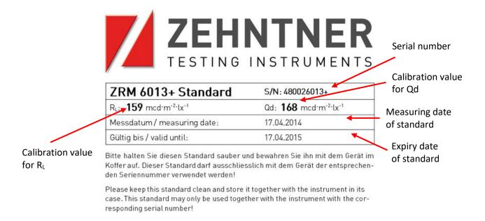
After the expiry date of the calibration standard a factory calibration of the ZRM 6013+ and its corresponding calibration standard is required. Contact either Proceq or your authorized Proceq-agent.
