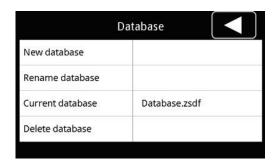
Here you are able to choose your desired database, rename a database and delete a database which is no longer used. Sometimes it is helpful to store all measurements for a specific project in a new database.
