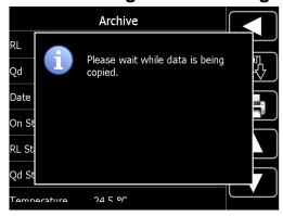
connect a USB-stick on the USB-interface (host). By pressing the button all measuring entries will be stored on the USB-stick. The message beside will be shown during copying. The exported measurements can be opened on a computer/laptop using the mapping software "MappingTools". The Use of MappingTools is described in the separate instruction manual.
