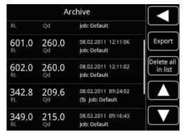
In the first column you see the  $R_L$ -values and in the second column the Qd-values. In the third column there are listed the date, time, the number of single measurements e.g. (5) at average measurements as well as the job. Press on a desired line for getting some additional information to the entry.
