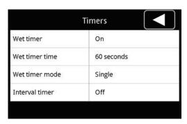
If the wet timer is activated, you can see the current setting for the wet timer time and wet timer mode. For changing these settings, you need to press on the respective line.
