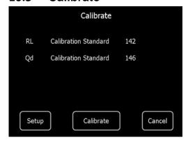
Press the symbol and to open the calibration function. In the standard setting there are listed night visibility RL and day visibility Qd to be calibrated on
