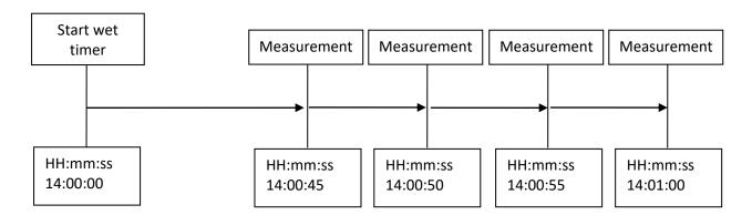
The first measurement will be carried out by the wet timer. Afterwards the set number of interval counts will be carried out. So in this sample there will be altogether 4 measurements.
