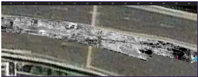
Interface defects between Asphalt-to-Concrete (A/C) layers (Delamination.)
